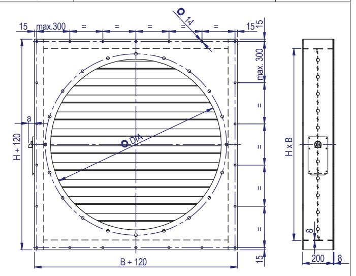
NYBORG RECTANGULAR SHUT-OFF DAMPER, DESIGNED FOR CIRCULAR APPLICATION, SSVent BxH, made of hot dipped galv. Steel. Damper blades and shafts in AISI 316L. Adapterplate is made of hot dipped galv. steel. Equipped with electrical or pneumatical actuators.
